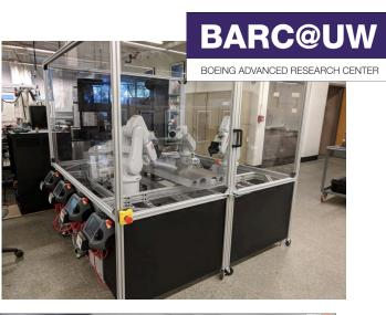
Robots Kenny, Kyle, Cartman and Stan drill and fasten a wing panel.
